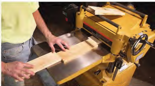
The planer train. When planing short stock, you should always butt the ends of the boards against one another as you feed them into the machine. This will reduce kickback and snipe.
